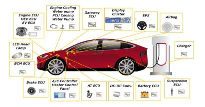
Power train: Engine control / Transmission control/ Idling Stop System / EV motor control etc... Chassis: ABS / ESC / EPS / Steering lock / Suspension etc... Body: Airbag etc...
